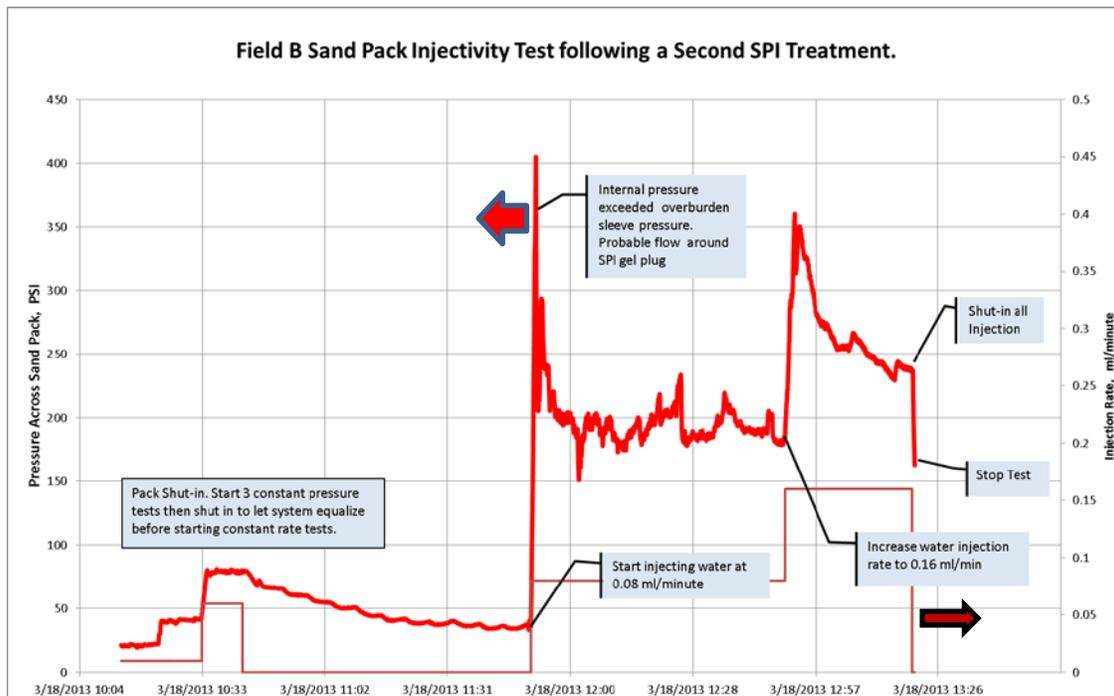
Figure 26. Water Injectivity re-Test of Field B Dolomite Sand Pack with early Constant Pressure Period before Constant Rate, following 2<sup>nd</sup> SPI Treatment.
