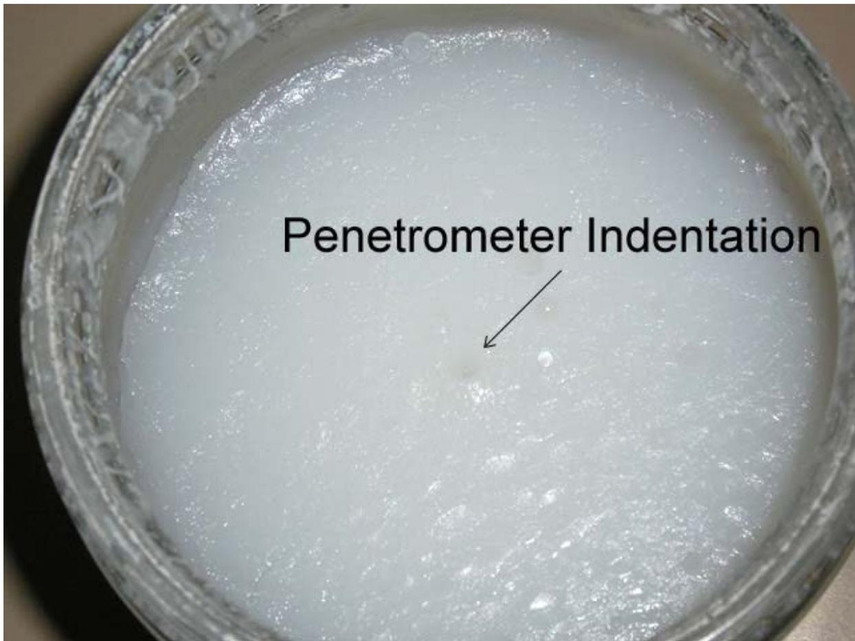
Figure 19. Penetrometer Test on an SPI gel
