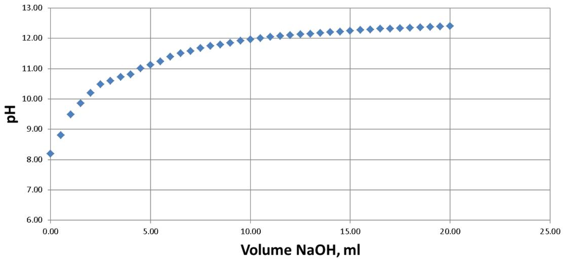
Figure 16. Titration with 0.1M NaOH into 100 grams of Field A Brine
