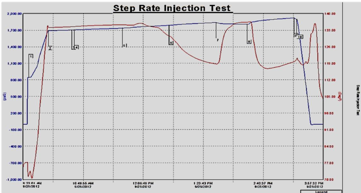
Figure 47. Field A, Well #2's (Production Well) pre-SPI Treatment Water Step Rate Test with bottom-hole pressure/ temperature bomb/ sensor.
