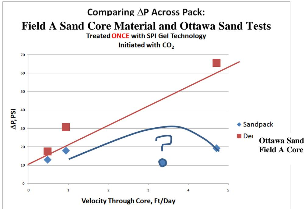
Figure 24. Field A Sandstone and Ottawa Sand Pack Water Injectivity Tests after 1<sup>st</sup> SPI Treatment
